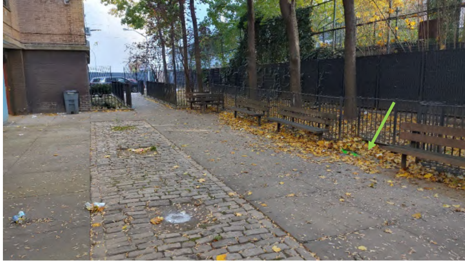
Photo 2 – Area located behind the building on site. The white circle shows a proposed soil boring location, while the green arrow shows the location of a partially covered storm drain. The storm drain line extended away from the area of concern towards the parking lot in the background.
